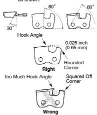
warning: Maintain the proper hook angle according to the manufacturer's specifications for the chain you are using. Improper hook angle will increase the chance of kickback which can result in serious injury.
